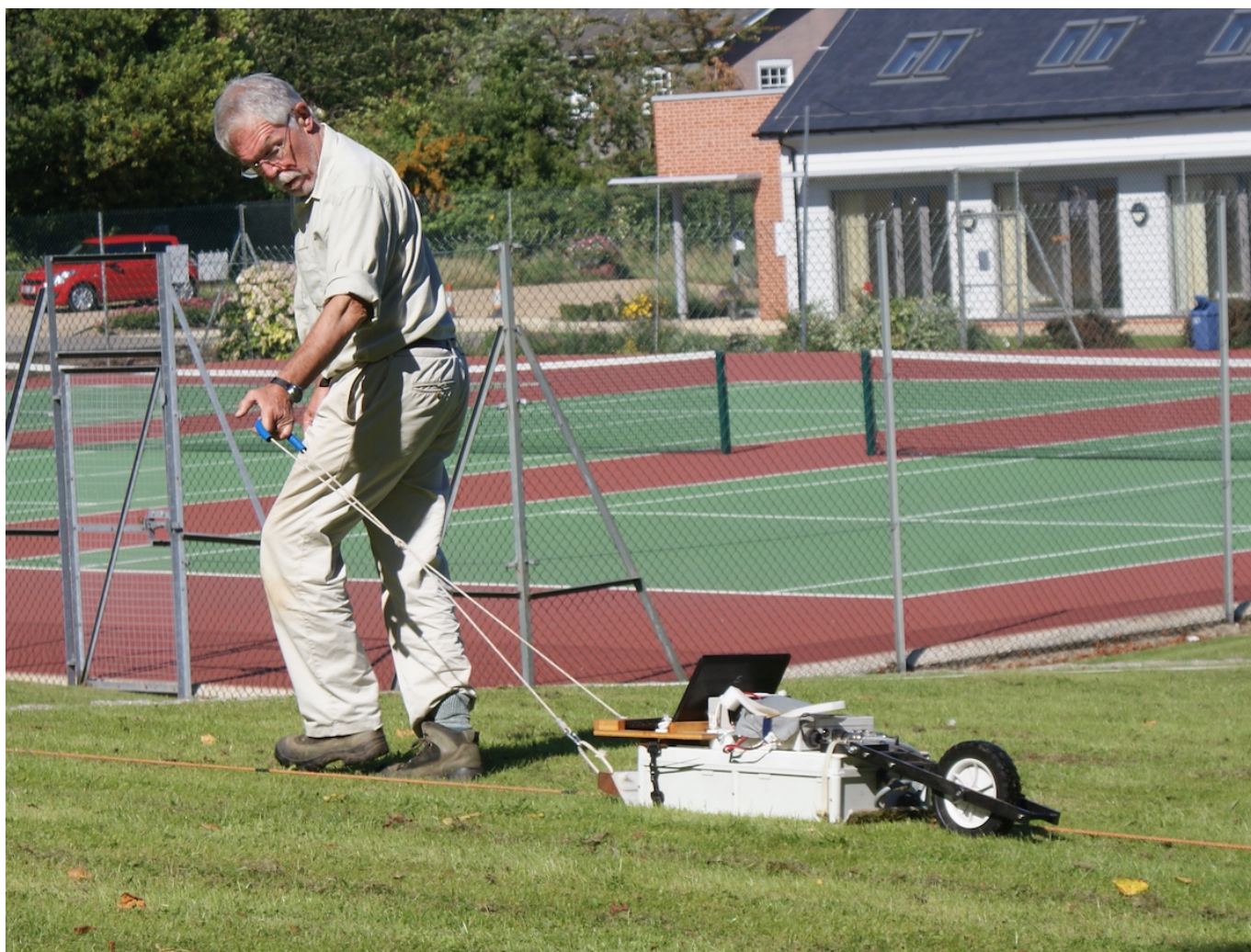
Figure A2. GPR survey in progress.
