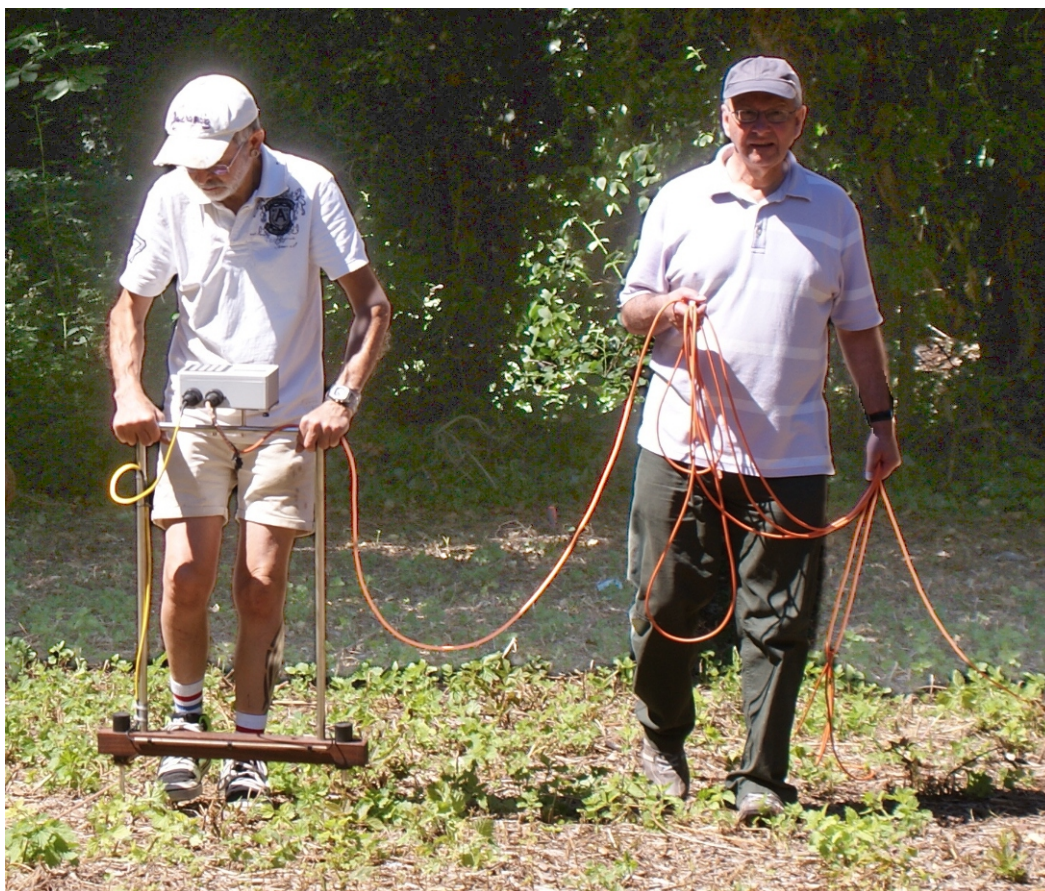
Figure A1. Ground resistance survey in progress.
