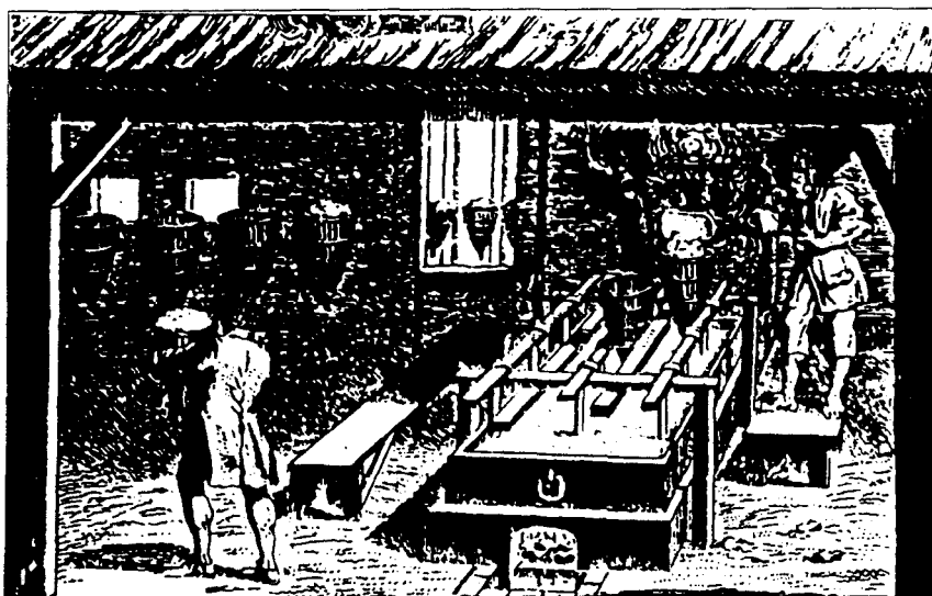
Figure 1) An 18 th Century Saltern. Excess brine from wet salt in the conical baskets drains back into the pan. A heated store in the background completes the drying process.
