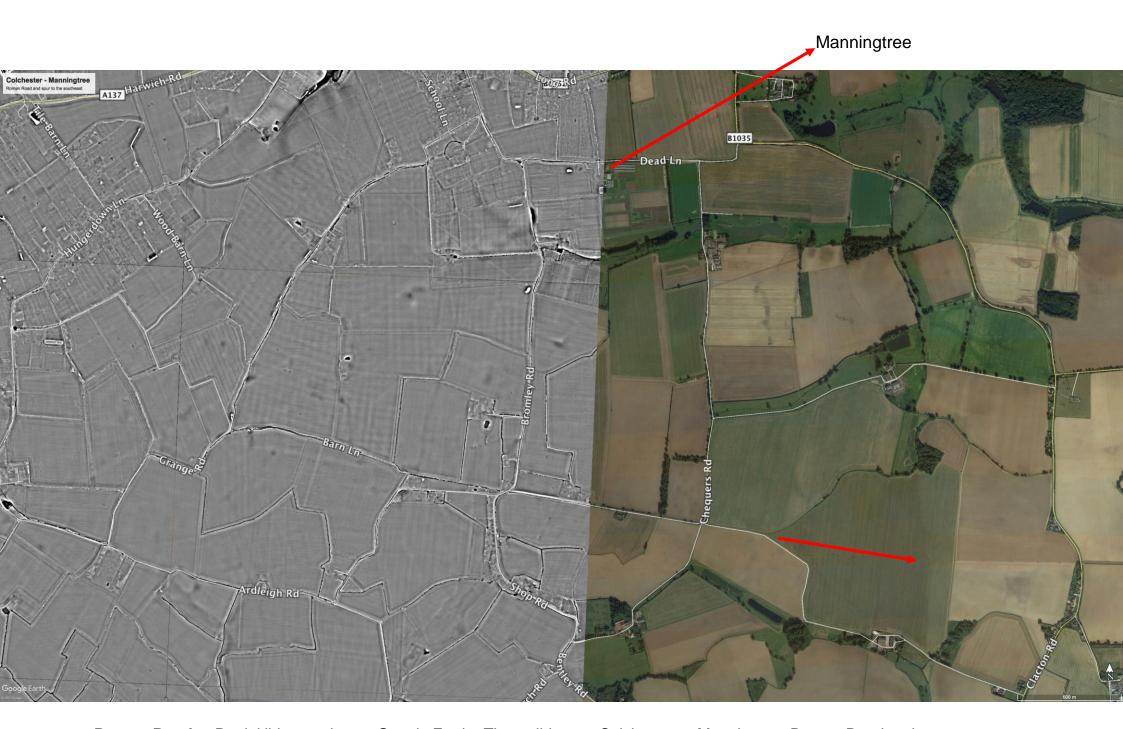
**Roman Roads**. Partial lidar overlay on Google Earth. The well-known Colchester to Manningtree Roman Road and a spur heading east towards Horsleycross Street, showing as faint light grey lines. A section of the spur is still followed by a modern lane.
